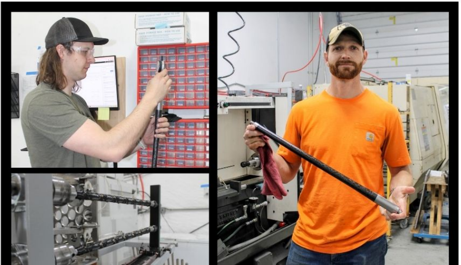
Clockwise from top left: Production Manager Cole Zacha carefully checks barrel land/groove measurements, ensuring they're within .0001 tolerance. Mike Johnson with a completed carbon barrel, and two rifle barrels in a "filament winding machine" that adds to the carbon's durability.
