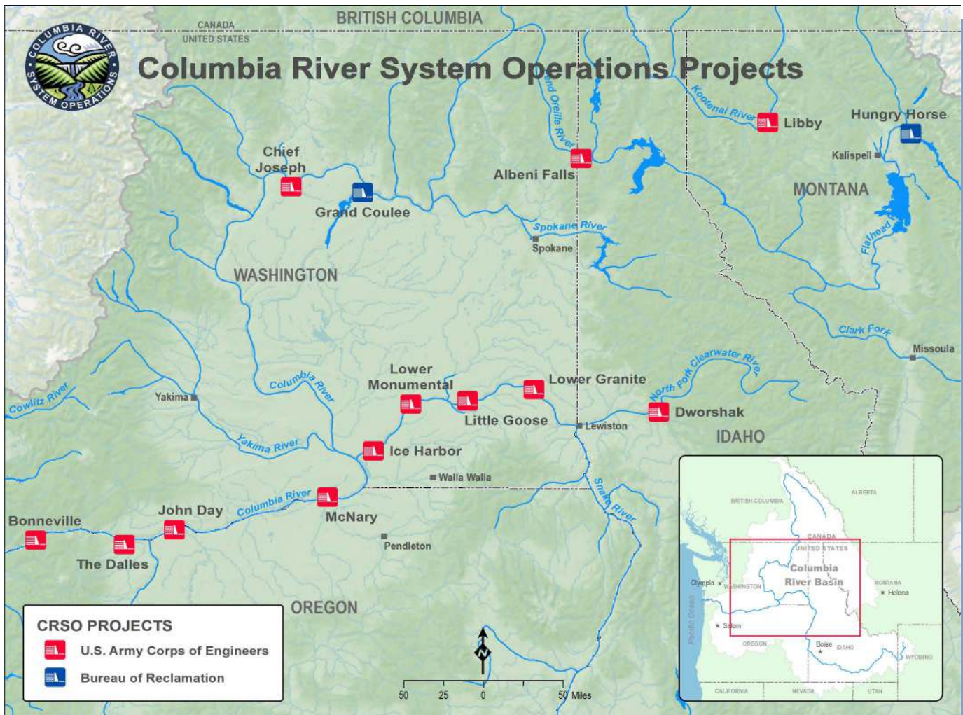
CRSO EIS water-quality modeling data is measured at the 14 system projects and other key locations in the Columbia River basin. Collected every 15 minutes, data includes water temperature, total dissolved gas, barometric pressure, flow, elevation and depth information from above and below these fixed monitoring locations.
