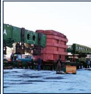
A BPA transformer, weighing approx. 320,000 lbs. and measuring 26' x 12' x 16.5' was transported by Union Pacific into town via the Port's rail line in early January. Omega Morgan is handling logistics to move the transformer to the Hatwai Substation near Genesee. Transformers convert high voltage electricity from power sources into lower voltage for use in businesses and homes.
