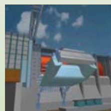
Spillway weirs at Ice Harbor, Lower Granite and Lower Monumental Dams are designed to be 'removable,' by controlled descent to the bottom of the dam forebay. This capability permits the spillway to perform to its original flow
